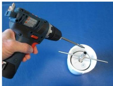
5. Remove the power drill and the magnetic bit extension. Remove the Key by unscrewing it from the Plug’s thimble. Replace the plastic center cap. Replace the cleanout’s standard cover to prevent debris from filling the cleanout.
