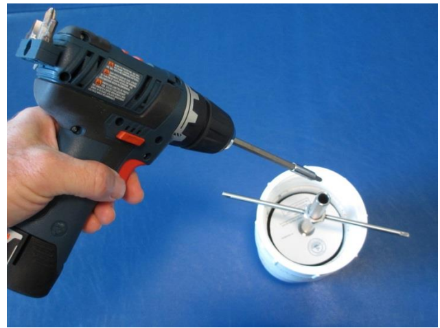
Fig. 2. Power Tightening with Keyed Torx Bit
